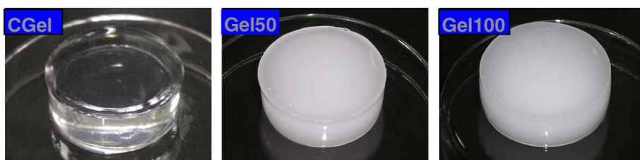
Fig. 1. Optical photos of the PNIPAAm hydrogels prepared in pure water (CGel) and phenol aqueous solutions with different concentrations of 50 mM (Gel50) and 100 mM (Gel100).
